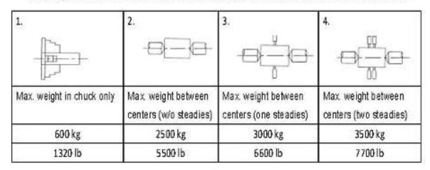
Max weight could bear for KL-3000 & KL-3200 Series (Ø155 mm Spindle bore x 350 mm Bed width)
