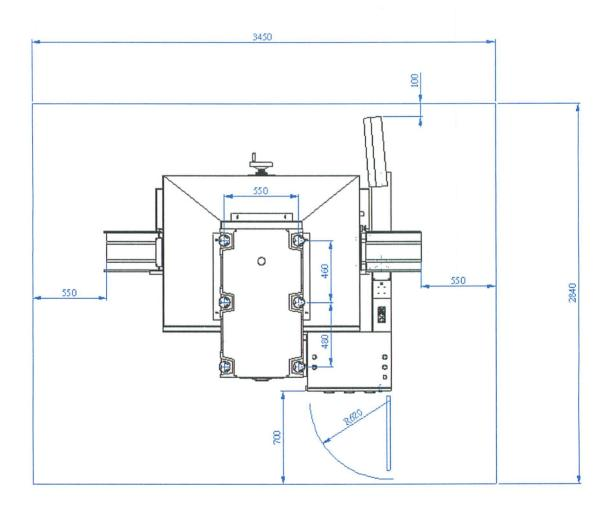
Machine floorspace required need 2700mm-2750mm
