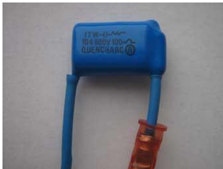
Figure 1, Pakron quencharc suppressor.
