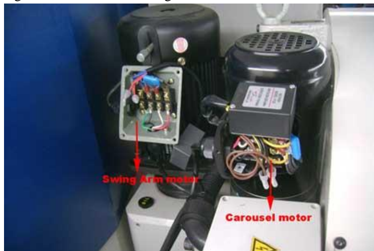
Figure 3, Overview of swing arm and carousel motor
