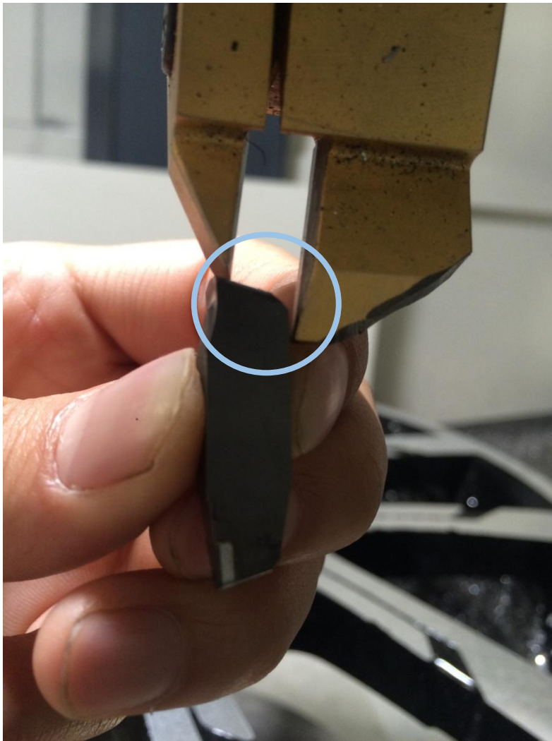
Step 3: Place new Diamond/Carbide insert into Tool Holder.
